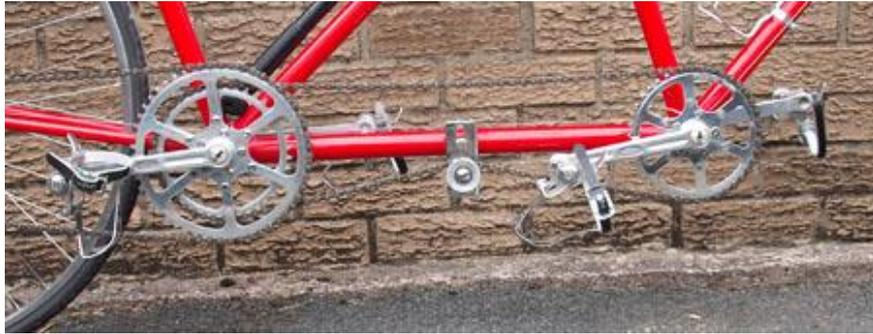
*Pennine tandem drive with two Stronglight.TA chainsets and Cyclo tensioner to take up chain slack between front and rear chainsets.*
