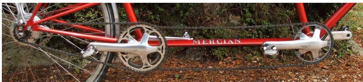
*In-line drive on this Mercian tandem with hub gears and rear disc brake*
