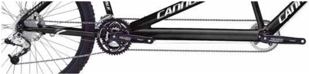
*Crossover drive on this Cannondale with derailleur rear, front triple changer and disc brake. As small chainring seems smaller than largest sprocket, lowest gearing must be about 20"*
