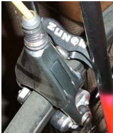
Zunow brake bridge on seat stays 'Just look at the dust on that brake'
